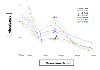
Figure:2 UV-vis spectra of silver nanoparticles at different concentration of silver ion
