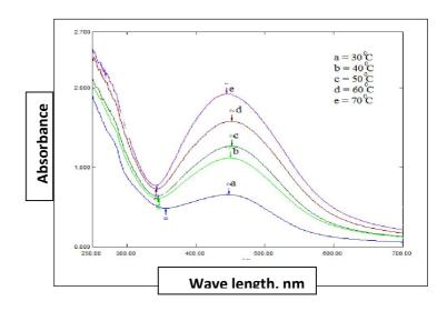
Figure:5 UV-vis spectra of silver nanoparticles at different Temp
