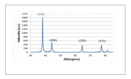
Figure:7 X-ray diffraction pattern of silver nanoparticles Prepared with *Carissa* extract
