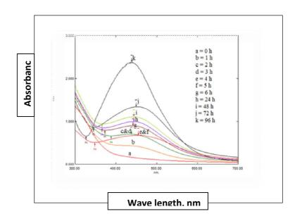
Figure:4 UV-vis spectra of silver nanoparticles at different contact time
