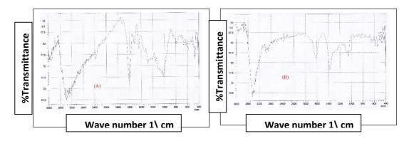
Figure: 6 FTIR spectra of capped silver nanoparticles
