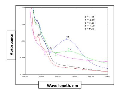
Figure: 3UV-vis spectra of silver nanoparticles at differentpH
