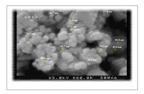
Figure: 8 SEM image of silver nanoparticles prepared with Carissa extract
